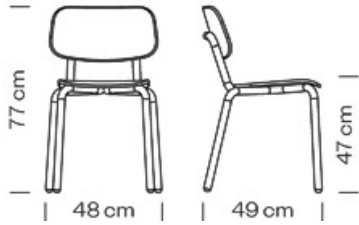
Chair with 4 legs steel frame. Beech wood seat and back (embossed finish).
