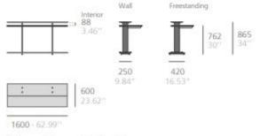
This module must be fixed to the floor or to the wall. Anchors included.
