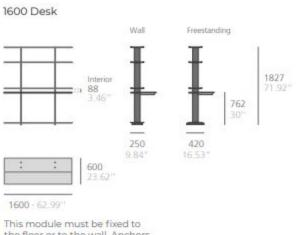
This module must be fixed to the floor or to the wall. Anchors included.
